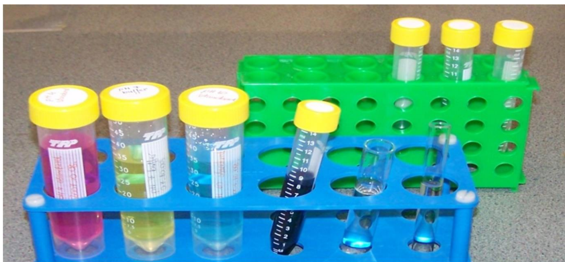
Figure (3.1) 50-mL and 15-mL Falcon tubes, glass test tube and Wasserman tube (left to right in blue rack) in plastic racks.
