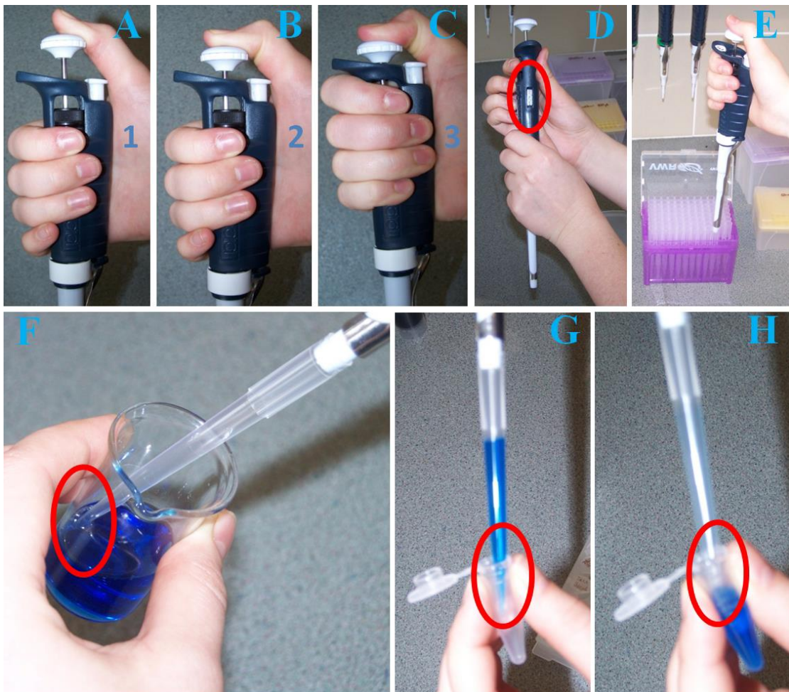
Figure 3.5 A-C, Three positions of the button of the pipette. D-H, Liquid handling with pipettes. D, Adjusting the volume. E, Fastening an appropriate tip. F, Drawing of the liquid. G, Transferring the liquid into an Eppendorf tube. H, Dispensing the liquid.
