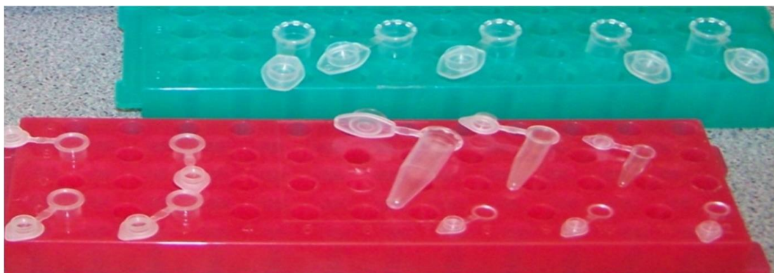
Figure 3.2 Eppendorf tubes with nominal volumes of 0.5 mL (left) and 1.5 mL (top green rack) and PCR tubes with a nominal volume of 200 \mu l (bottom right corner).
