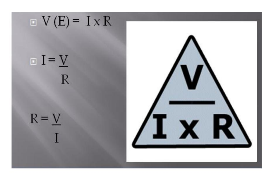
examp. What E is needed for a circuit with a R of 1.2K ohms and a I of .03 amps.
