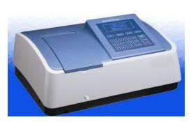
**Spectrophotometer** Is an instrument designed to detect the amount of radiant light energy absorbed by molecules.
