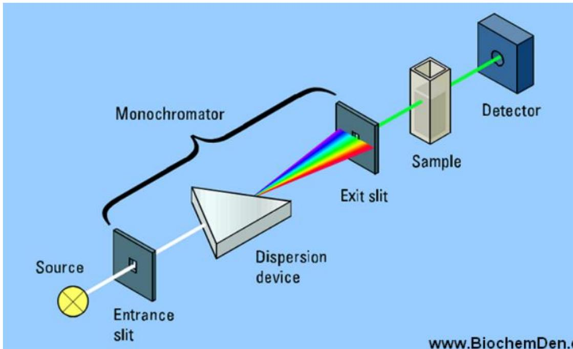
**Figure 1: Basic structure of spectrophotometers**
