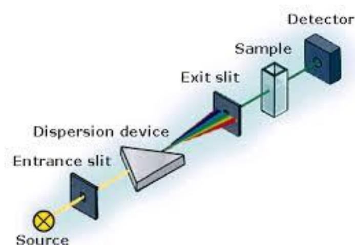
a) **Light source:** hydrogen lamp for U.V spectrophotometer and tungsten lamp for visible spectrophotometer.
