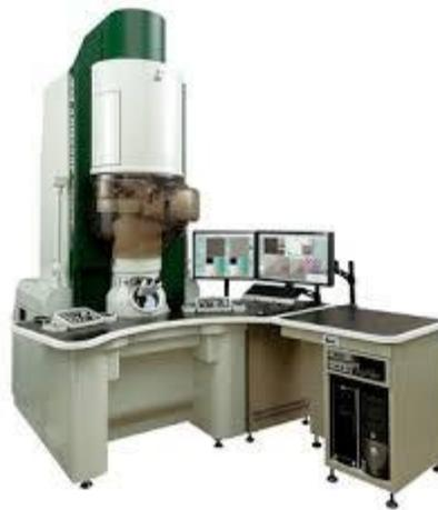
**Electron microscope (EM)** is a type of microscope that uses an electron beam to illuminate <sup>بيضيء</sup> a specimen and produce a magnified image
