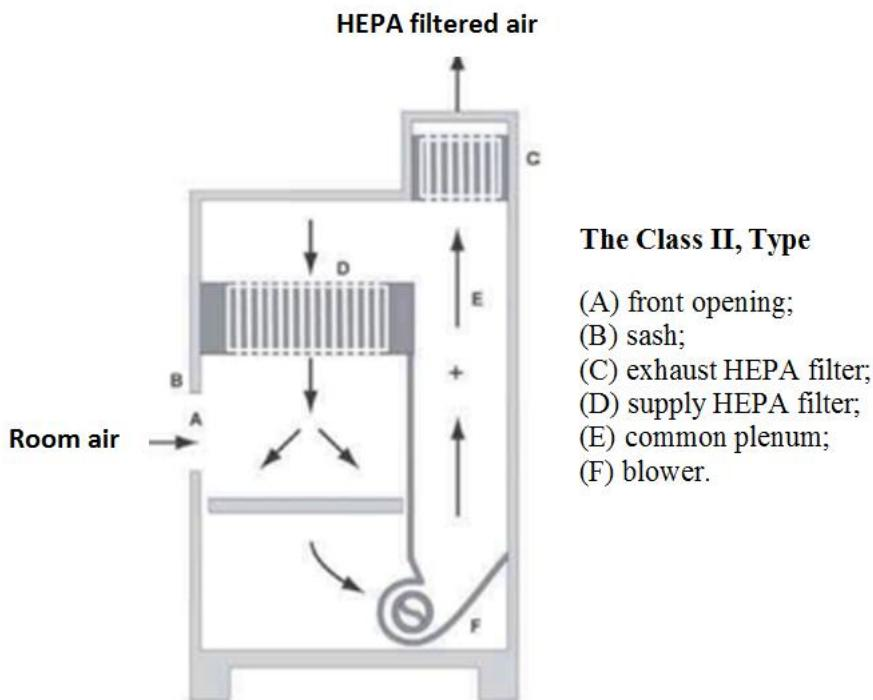
The Class 2 Biological Safety cabinet must meet the requirements for personnel, environmental and product protection. The air-flow is drawn into the work chamber via the front aperture and continues under the worktop and goes up the back plenum, where 70 % is being recirculated through the main triple HEPA filter to provide down flow and 30 % exits out through the HEPA filter to exhaust.
