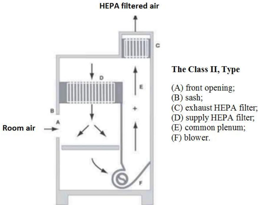
The Class 2 Biological Safety cabinet must meet the requirements for personnel, environmental and product protection. The air-flow is drawn into the work chamber via the front aperture and continues under the worktop and goes up the back plenum, where 70 % is being recirculated through the main triple HEPA filter to provide down flow and 30 % exits out through the HEPA filter to exhaust.
