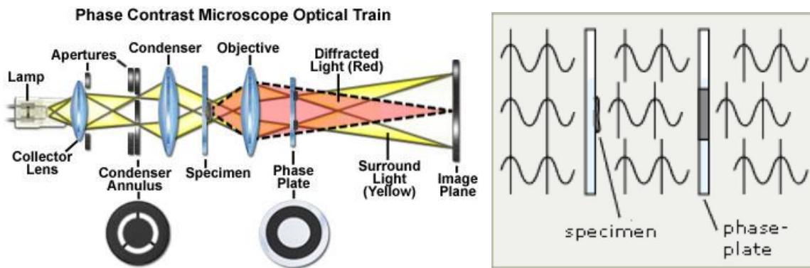
1. The phase contrast microscope uses the fact that the light passing through a transparent part of the specimen travels slower and due to this is shifted compared to the uninfluenced light.
