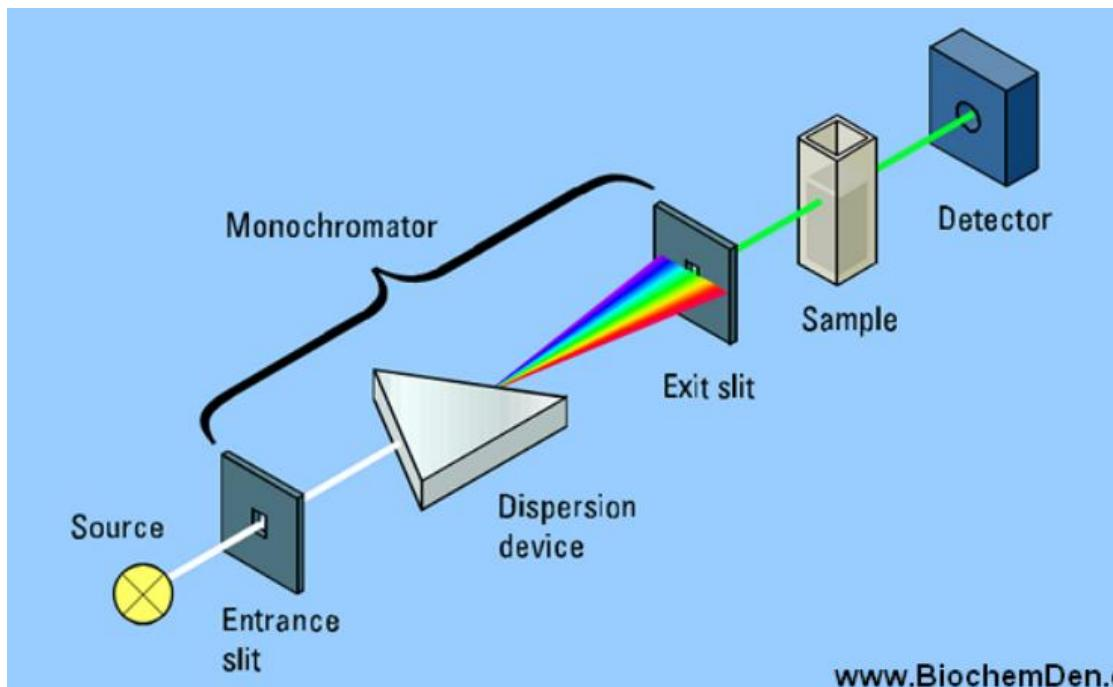
**Figure 1: Basic structure of spectrophotometers**
